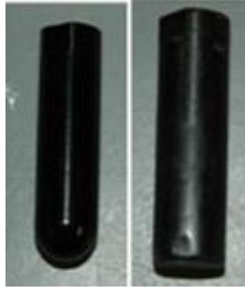
Figure 3.41: Tool Steel (left) and DELRIN® (right) Tup Insert (Zantout 2009)
