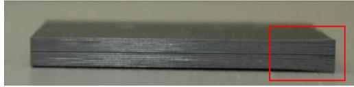
Figure 4.4: Corner Delamination in Side View of Cut Specimen 3
