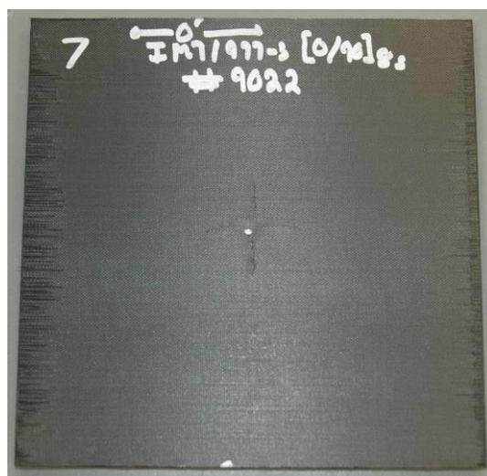
Figure 3.20: Impact Damage on the Top Surface of Specimen 7
