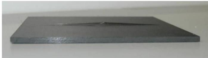
Figure 3.6: Side View of Impact Damage on the Bottom Surface of Specimen 2
