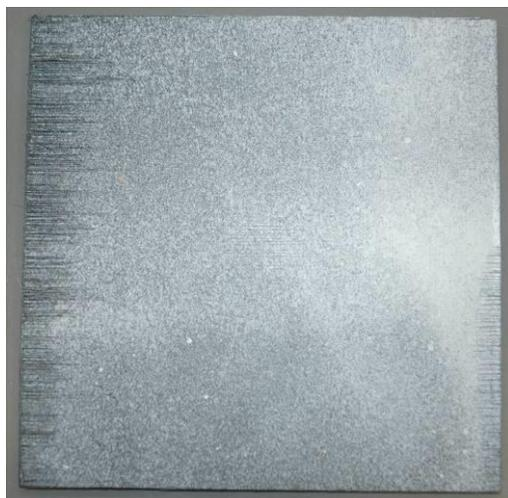
Figure 3.35: Impact Damage on the Bottom Surface of Specimen 11
